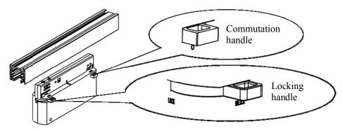
2. Align the protrusion of the rail light connector with the groove of the rail before assembly.
