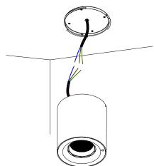
5. Align the clamp point on the lamp body with the hanging plate to avoid the opening, and tighten the lamp to the ceiling, as shown in the picture on the lower left.
