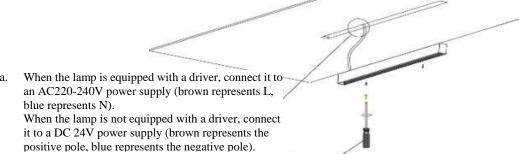
Align the installation holes with a screwdriver or electric tool, tighten the screws to secure the light fixture into the lamp slot.
