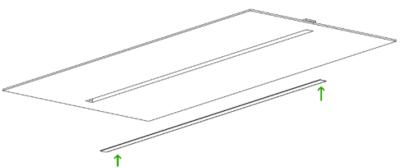
After fixing the lamp and lighting it up, confirm that the installation is correct Smooth buckle into the PC lampshade (To avoid splicing errors that may cause gaps in the lampshade after splicing, the equipped lampshade will be 1-2cm longer than the rated length. When splicing, cut off the longer section to achieve a no light leakage effect!)
