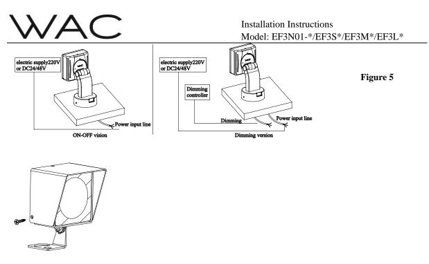
6. Installation of anti glare accessories for lighting fixtures (customer to purchase separately if necessary), fix the anti glare accessories to the lamp body with screws (see Figure 5).
