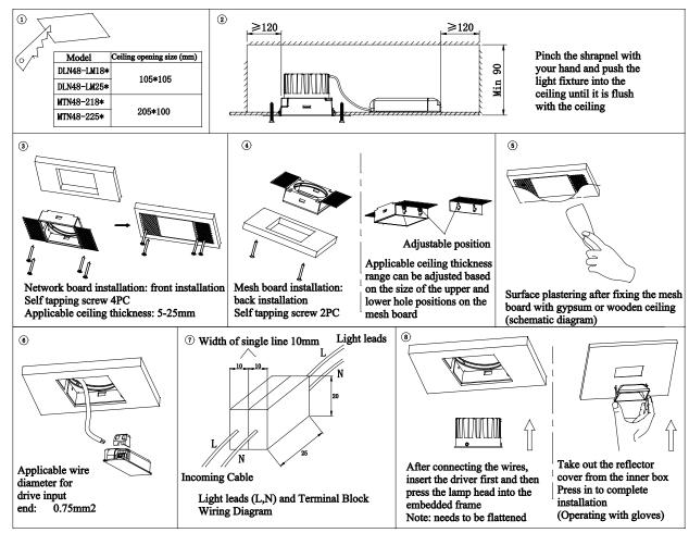
\*If the driver of the lamp comes with a lead wire, and this connecting lead wire needs to be connected to an independent terminal block(refer to the schematic diagram in Figure 7 for wiring, this lamp does not include this terminal block), the size of each terminal block should not be less than  $10\times20\times25$ mm.
