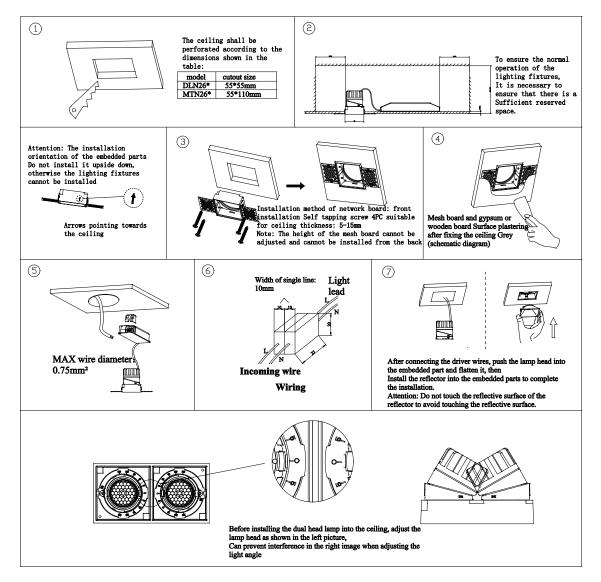
\* If the driver of the light comes with lead wires, and the leads need to be connected with an independent terminal block (refer to Figure 3 for wiring), the size of the terminal block for each line should not be less than 10x20x25mm.
