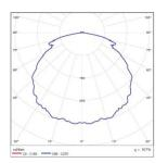
MODEL: ED310-15MT-130TC BEAM / ANGLE: / POWER: 0.3W LUMENS: 7 lm CBCP: / EFFICACY: 26 lm /W
