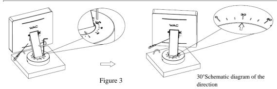
4. Vertical adjustment of the lamp from 0 °to 90 °(counterclockwise). The corresponding angle of the rotating lamp body is aligned with the scale mark of the lamp body support arm, the fastening screw (tool 4.0mm hex wrench) on the lamp body is locked in a clockwise direction, release the adjustment in the opposite direction (as shown in Figure 4);
