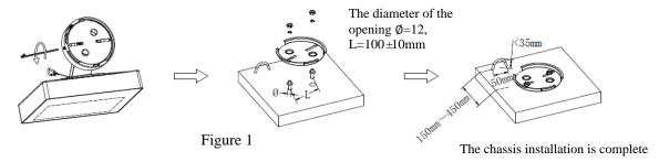
2. Thread the lamp cable out of the cable of the installation chassis
