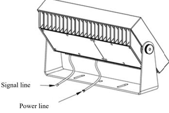
3) Match and connect each core wire of the lamp to the power input (220V/AC), and the monochrome non dimming version does not have a signal wire.
