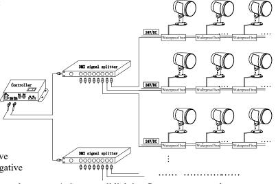
4. Connect all lighting fixtures to a control network and adjust control as needed
