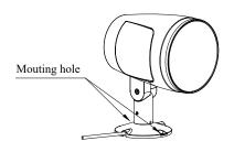
1. Fix the light fixture with appropriate screws through the installation holes shown in the diagram
