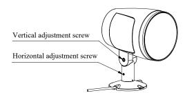
2. The lamp can be rotated horizontally by 330 degrees using an Allen wrench, and vertically by 30 degrees in the front and 90 degrees in the back to adjust the direction
