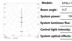
Models: EP5LI-108EL-V30BK  $4.2^{\circ}$ Beam angle: System power: 108W (Max) System luminous flux: 6379lm **Central light intensity:** 56.65lm /W
