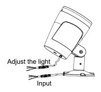
4. Dimming version has two lines, please follow the instructions on the label wiring, wiring waterproof treatment
