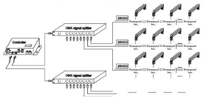
**Note:** The wire connection must use a waterproof junction box with an IP65 or higher rating, and the waterproof joints of the junction box must match the leads of the lighting fixtures. It is recommended that the total length of the splicing of the lighting fixtures connected to each power circuit should not exceed 14 meters, and it is advisable to have no more than 32 lighting fixtures carried by each DMA signal amplifier.
